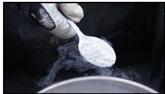
Figure 2: Icy-regolith sample with 5% ice mass content.
